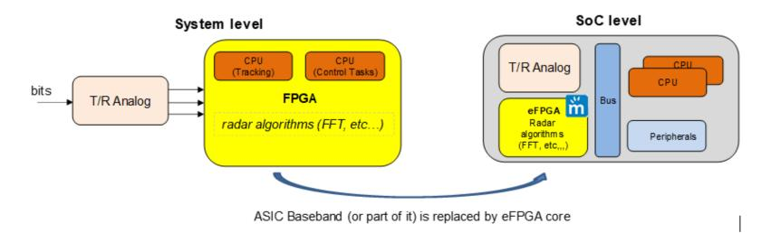
It improves also performance in term of Image Processing thanks to eFPGA dedicated blocks like complex DSP for FFT computing, complex multipliers and FIR Filters.
