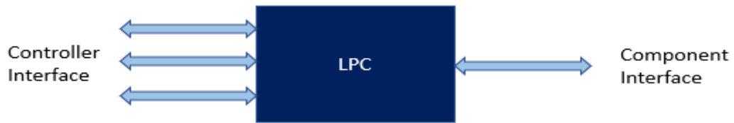
Figure 5 Low Power Combiner
