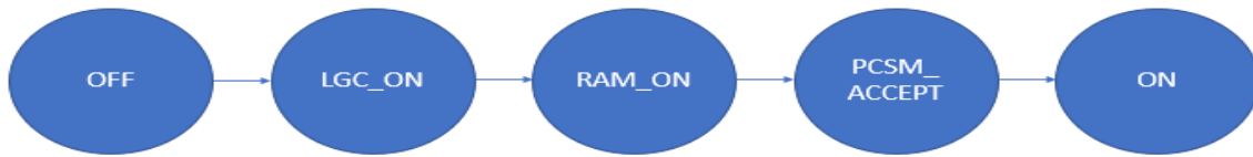
Figure 3: PCSM Power Mode Transitions Sequence
