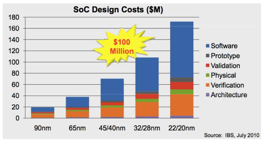
Mask costs: ~\$1M for 40nm, ~\$2M for 28nm, ~\$5M for 16/14nm! Engineering cost/complexity shifting full custom to high level design
