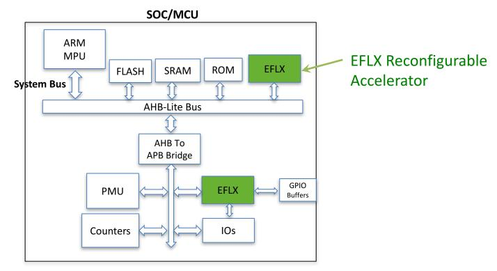
eFPGA accelerates AES/SHA/JPEG/FFT 30-140x faster than ARM
