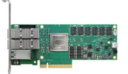
**Mellanox BlueField 2:** Software programmable Smart NICs. Combines embedded high-performance 64-bit processors (8 to 16 x 64-bit ARM cores) and performance optimized offload accelerators for network and application layer functions.
