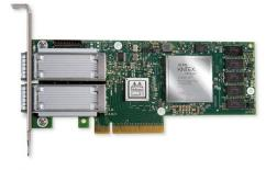
**Mellanox Innova II:** Semi-programmable Smart NICs. Combines highly efficient standard NIC technology with programmable logic for customization of critical network and application layer functions.
