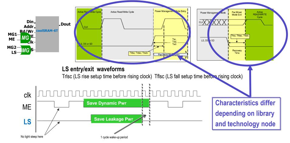
PowerPro Memory Gating insures "Light Sleep" (LS or TLS) signal meets Trlsc and Tflsc requirements
