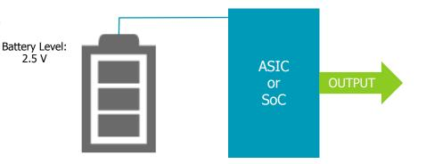
The Flexsupply<sup>™</sup> family of switched-capacitor regulated voltage-doubler IP cores are designed to improve current products so that they can function properly at extremely low battery levels.
